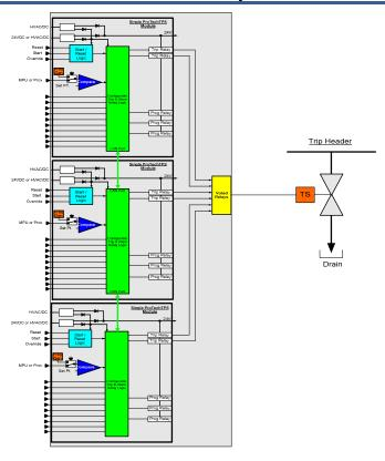
Figure 3-6. Simplex Trip Block Assembly
