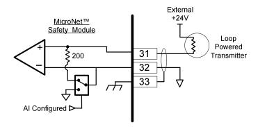
Figure 2-14. Example Configurable Input Wiring—Analog Input
