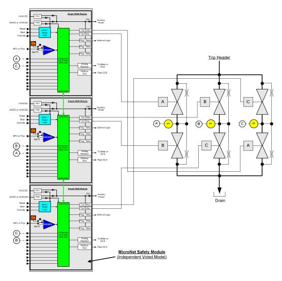
Figure 3-3. Example TMR Trip Block Assembly Interface
