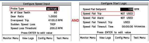
Figure 5-1. Configuration Guide - Front Panel Interface with Active Probe
