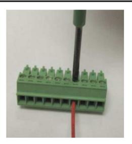
Torque range for screws of Screw Connection Terminal Blocks: (0.22–0.25) N⋅m / (1.95–2.21) lb-in
