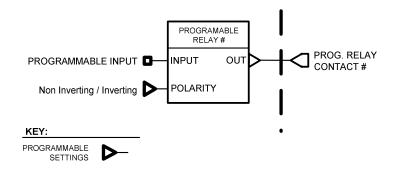
Figure 3-10. Programmable Relay Output Diagram
