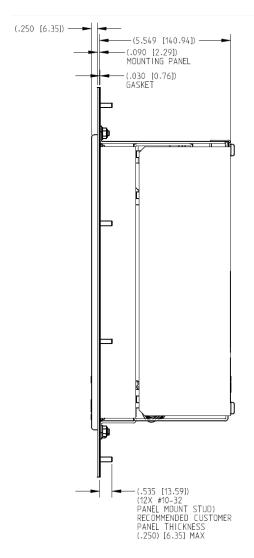
Figure 2-5b. Mounting Outline Diagram for Panel-Mount Models
