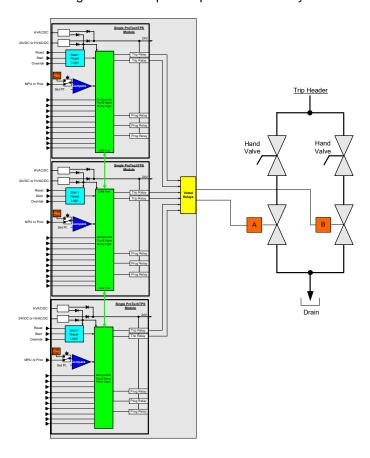
Figure 3-7. Dual Redundant Trip Block Assembly
