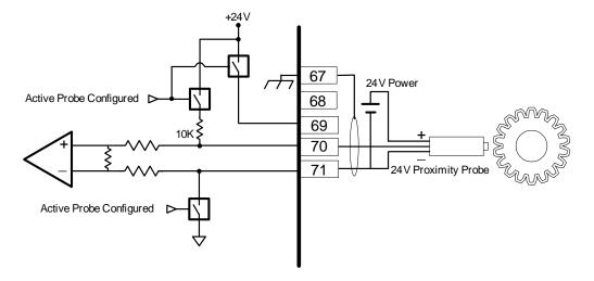
Figure 2-11c. Example Proximity Probe (Active Magnetic Pickup Unit)
