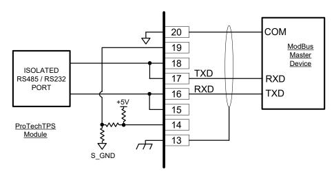
Figure 2-18a. Serial Port Interface Diagram—RS-232
