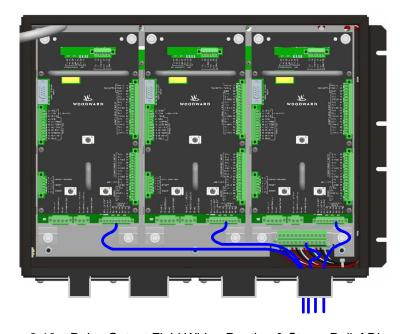
Figure 2-10c. Relay Output Field Wiring Routing & Stress Relief Diagram
