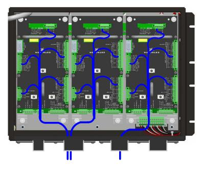
Figure 2-10b. Configurable I/O Wiring Routing & Stress Relief Diagram
