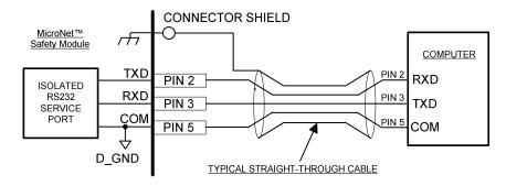
Figure 2-19. Service Tool Cable/Interface Diagram
