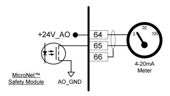
Figure 2-15. Example Analog Output Wiring
