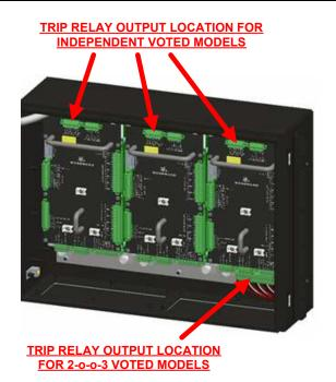
Figure 2-16a. Example Trip Relay Output Wiring
