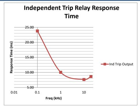
Figure 3-15. Independent Trip Relay Response Time (Typical) Graph
