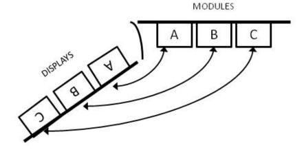
Figure 2-2a. Bulkhead Schematic Showing Front Panel A Connection to Module A and Front Panel C Connection to Module C—Top View
