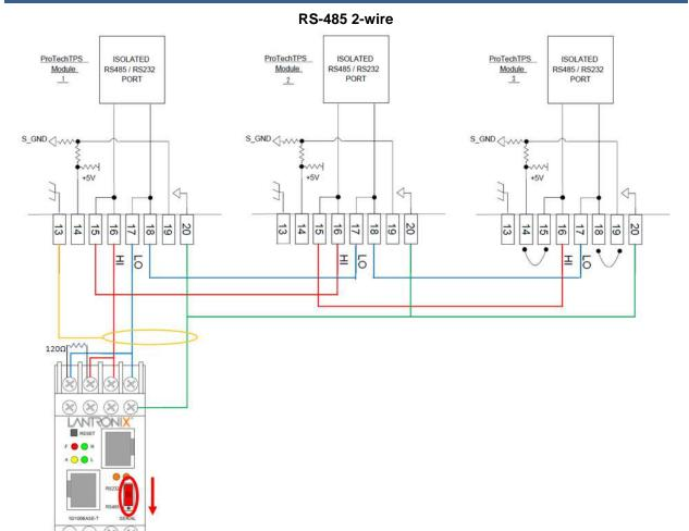
Verify that the dip switch on the front of the device is in the down position, indicating RS-485 communications. When configuring for RS-485, termination resistors (120  $\varsigma$ ) are needed at each end of the network. Note the location of the resistor on the device. The ProTech has the termination resistor built into the module, jumpers are necessary between terminals 14 – 15 and 18 – 19 to activate the termination.
