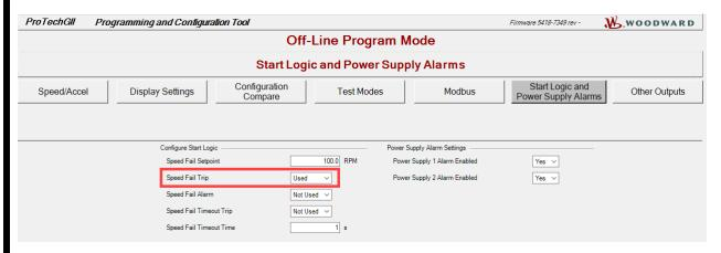
Figure 5-2. Speed Fail Trip Using PCT
