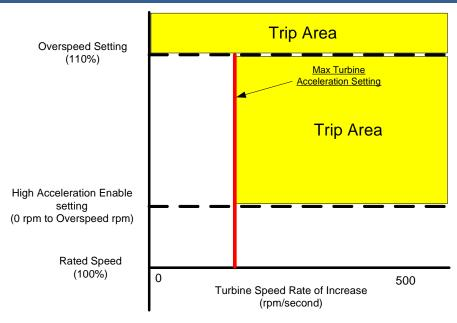
Figure 3-11. Over-Acceleration Enabling Diagram
