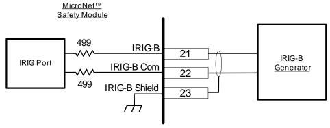
Figure 2-20. IRIG-B Interface Diagram
