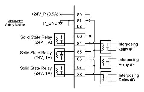
Figure 2-16e. Example Programmable Relay Wiring (Internal Supply)
