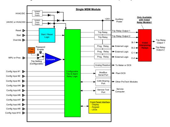
Figure 3-5. Functional Diagram of Single MicroNet Safety Module with Voted Trip Relay Outputs
