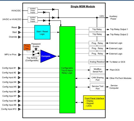
Figure 3-2. Functional Diagram of single MicroNet Safety Module with Independent Trip Relay Outputs
