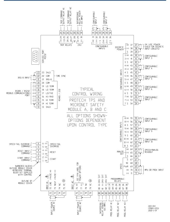
Figure 2-8. MicroNet Safety Module Control Wiring Diagram
