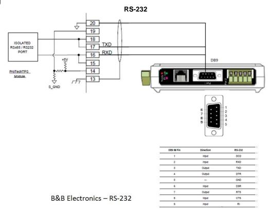
Note: The Serial DB9 connection is used for RS-232 communication only.
