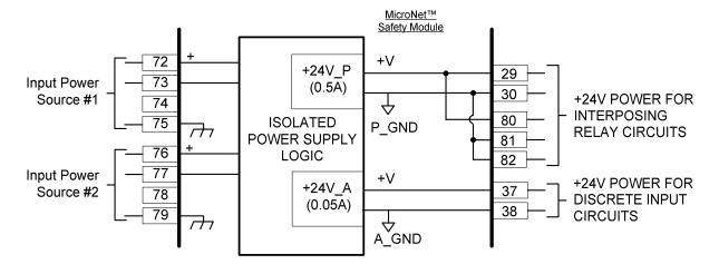
Figure 2-17. Power Supply Relationship Diagram
