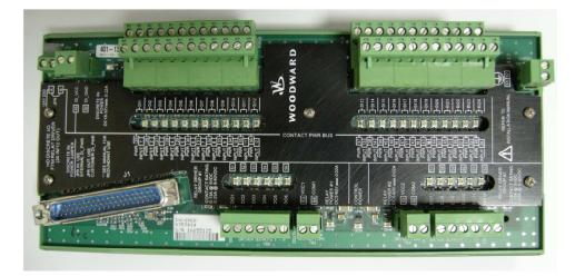
Figure 12-49. 24/12 Discrete I/O (with LEDs) FTM
