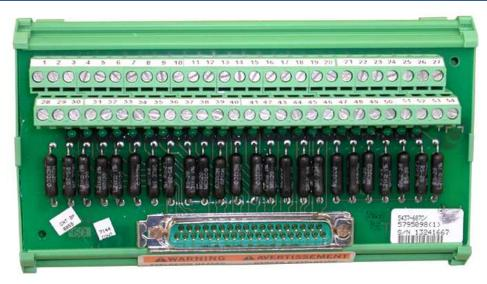
Figure 12-46. Discrete Input (with LEDs) FTM
