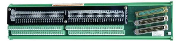
Figure 12-40. 24 Vdc 48/24 Discrete FTM
