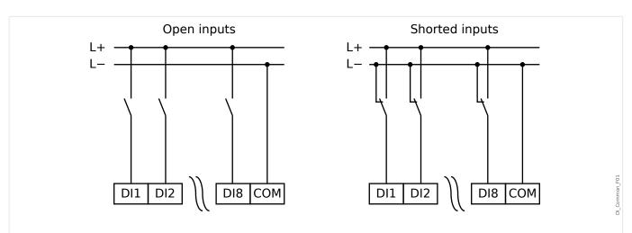
*Fig. 105:* Safe State of the Digital Inputs
