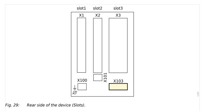
The data communication interface in the **X103** slot is dependent on the ordered device type. The scope of functions is dependent on the type of data communication interface.
