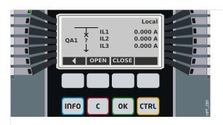
*Fig.* 87: Control Page Example, with the "Circuit Breaker" in faulty (or implausible) position.
