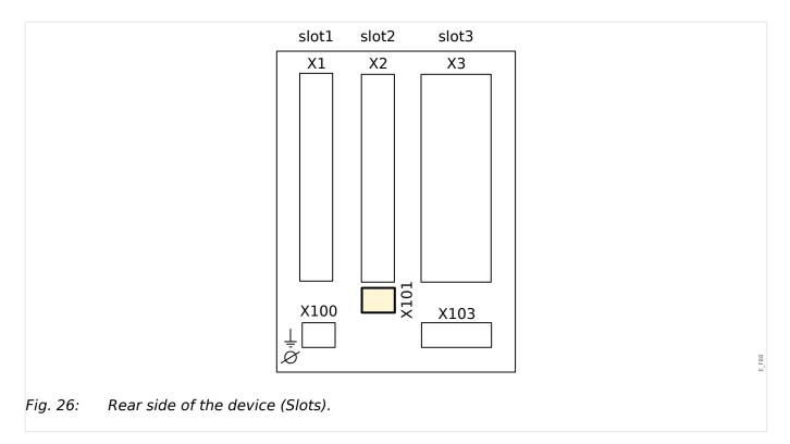
Depending on the ordered device type, this slot can be equipped with an IRIG-B interface.
