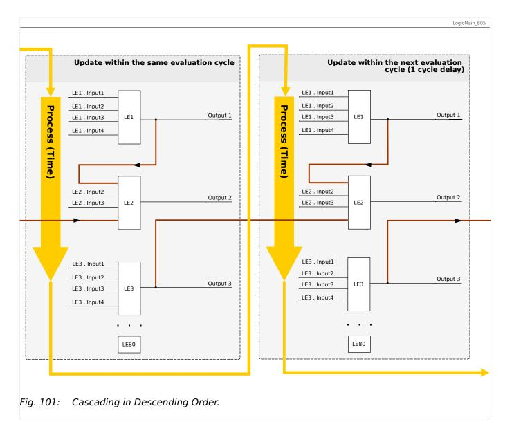
In the example shown in  $\sqsubseteq$  Fig. 101 above, "Logic Equation **2**" uses the output states of two other equations, "Logic Equation **1**" and "Logic Equation **3**". The result of "Logic Equation **1**" is used in ascending order and has therefore been evaluated within the same process cycle. The result of "Logic Equation **3**" is used in descending order and has therefore been evaluated in the previous process cycle.
