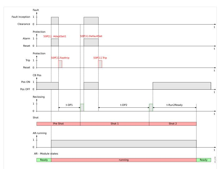
*Fig. 76:* Auto Reclosing timing diagram for **successful** 2-shot auto reclosing scheme with acceleration at pre-shot.
