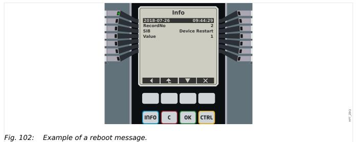
The reason for a device start/reboot is shown numerically as "Value". The value "1" in the example above means a normal start-up. Please see the table below for a full list.
