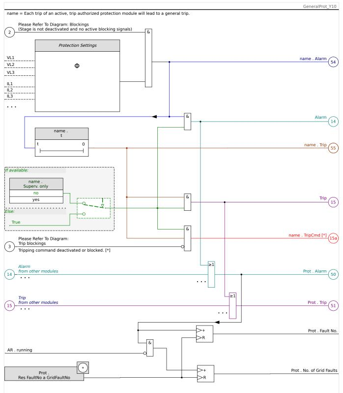
*Fig. 43:* Rough sketch of the functionality of any HighPROTEC protective element.
