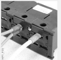
Remark: As long as the cable cross-sections are within the limits given in the Technical Data chapter ( 4 > 12 Technical Data", L Table ) it is also possible to insert two rings into one terminal, as shown here. This is useful for setting up the neutral point connection.
