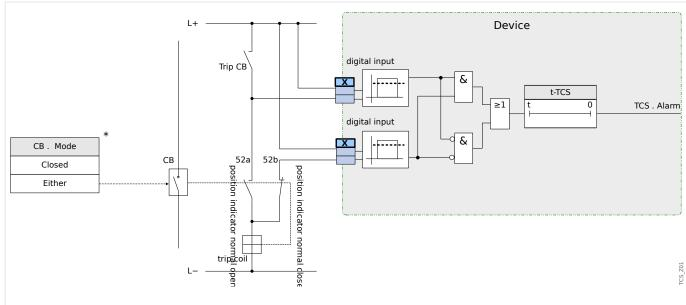
Fig. 83: Connection example: Trip circuit supervision with two CB auxiliary contacts »Aux ON« (52a) and »Aux OFF« (52b).
