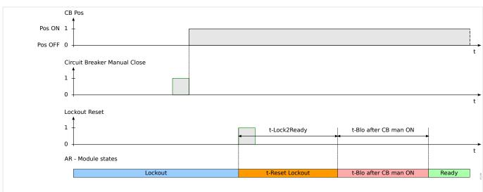
*Fig. 80: AR Lockout Reset Logic in case lockout Reset coming after manual breaker closed.*
