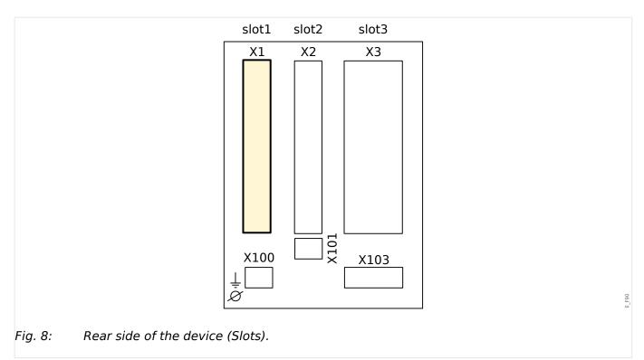
The type of power supply card and the number of digital inputs on it used in this slot is dependent on the ordered device type. The different variants have a different scope of functions.
