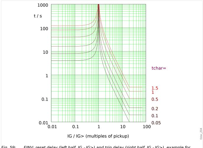
*Fig.* 59: EINV: reset delay (left half, IG < IG>) and trip delay (right half, IG > IG>), example for  $I_{G,max} = 20 \cdot IG>$ .
