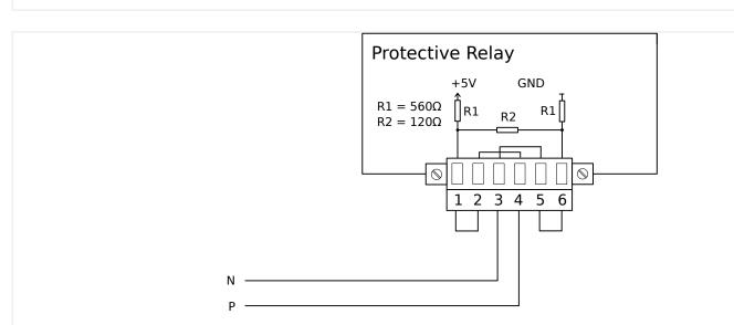
*Fig. 33: Wiring example, Device at the end of the bus. (Setting wire jumpers to activate the integrated Terminal Resistor.)*
