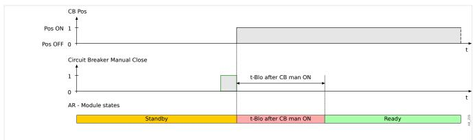
*Fig.* 77: Auto Reclosing States during manual breaker closing.
