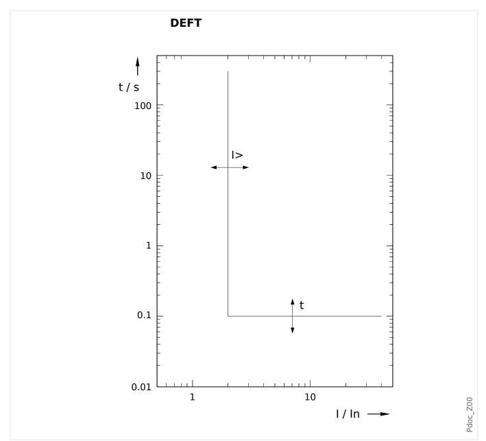
Trip delay for I > I>, settable via [Protection Para / Set 1...4 / I-Prot / I[x]]  $>t \ll$ . The reset delay for I < I> always equals 0 ("instantaneous").
